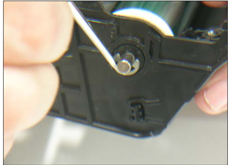
19. Remove the shaft of the drum by releasing the retaining washer from the left side of the cartridge.
